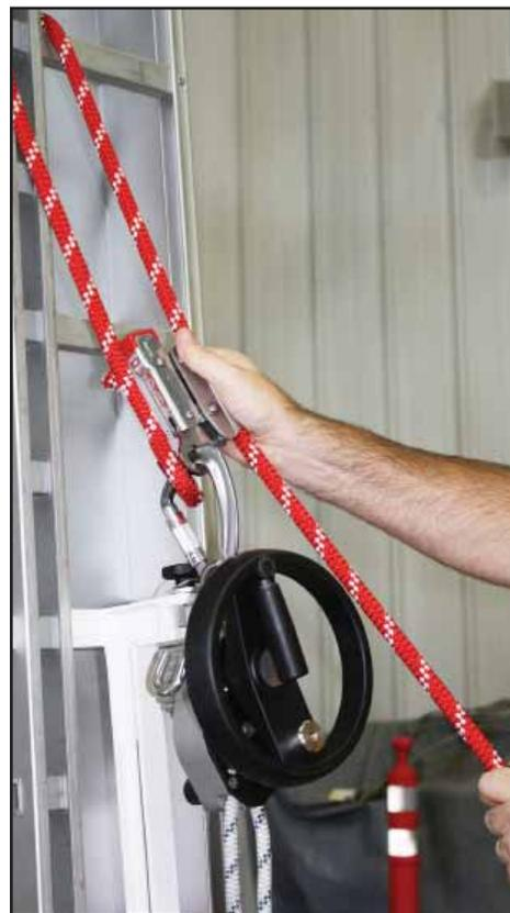
To remove the rope anchor, squeeze the rope grab to release the locking mechanism and loosen the rope. Then detach the carabiner and remove rope anchor from anchorage.
