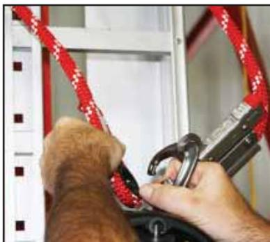
Step 1 - Wrap rope anchor around approved anchorage and attach locking carabiner through both the eye of the rope grab and the rope thimble. Ensure that the carabiner is completely closed and locked.
