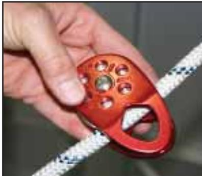
Step 1 - Rotate one half of the pulley to allow insertion of the lifeline. Once lifeline is inserted, return pulley to aligned position.
