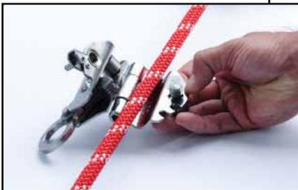
Step 1 - Open the latch and unscrew the locking thumbscrew to open the device. Place the device on the compatible rope lanyard with the arrow label on the rope grab pointing toward the anchor point.
