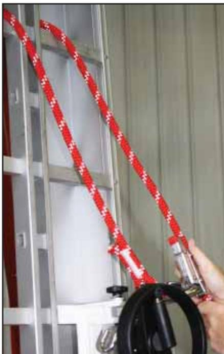
Step 2 - Push upward on the rope grab until the rope anchor is taut.
