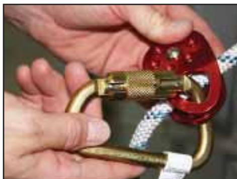
Step 2 - Attach locking carabiner to pulley. Ensure that the carabiner is completely closed and locked.
