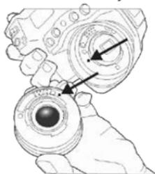
2. *Carefully push the lens into position.*
