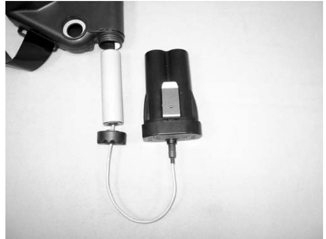
Figure 5. Alkaline Battery Pack Installation
