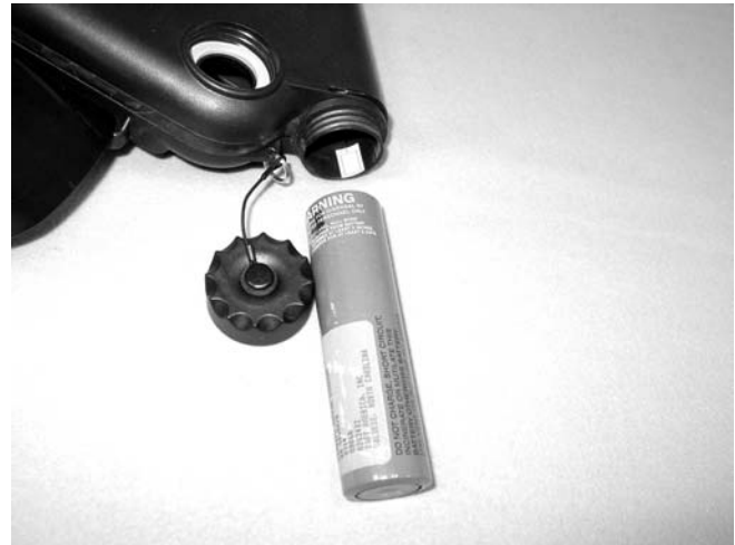
Figure 2. Non-rechargeable Li-SO 2 Battery Pack Installation
